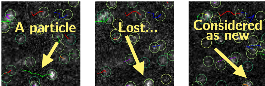
FIGURE 12. Example of a lost trajectory through three consecutive frames even though the signal was clear, such events have a tendency to provide wrong statistics (for instance, it divides molecule lifetime by roughly two each time a link is lost)
